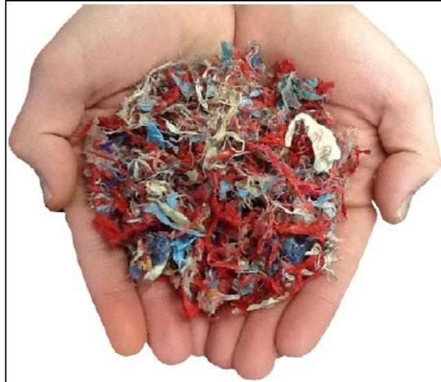
Colorado Medical Waste's ecofriendly process shreds medical waste to a confetti-like residual. The waste is sterilized and reduced in volume by 90%.
